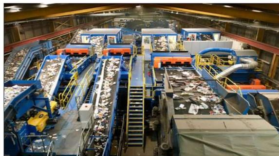
**Figure F 3.2a:** typical conveyor layout in waste treatment plant that requires protection under conveyors and platforms as well as protection under covered area, in addition to the ceiling protection.
