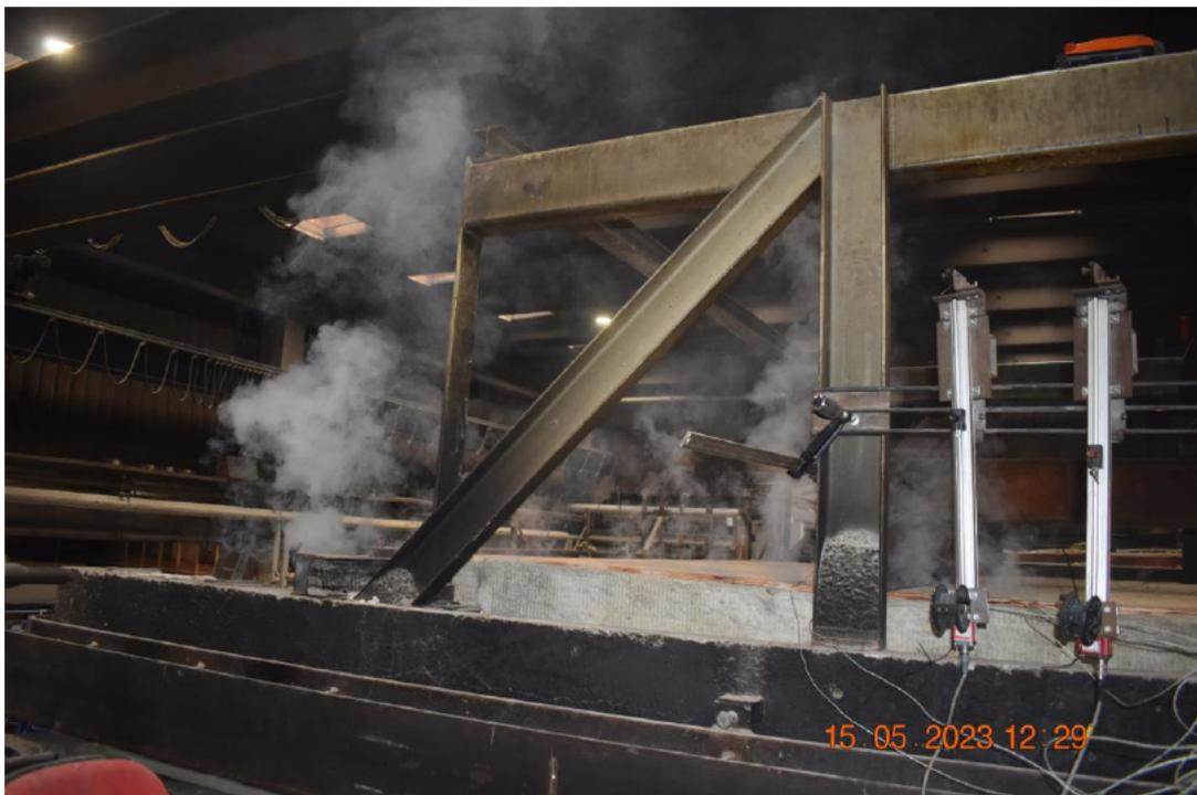
Photo No. 21 Test specimen seen from unexposed side 49 minutes into testing
