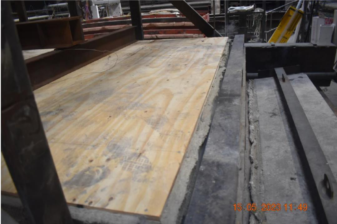
Photo No. 18 Test specimen seen from unexposed side 10 minutes into testing
