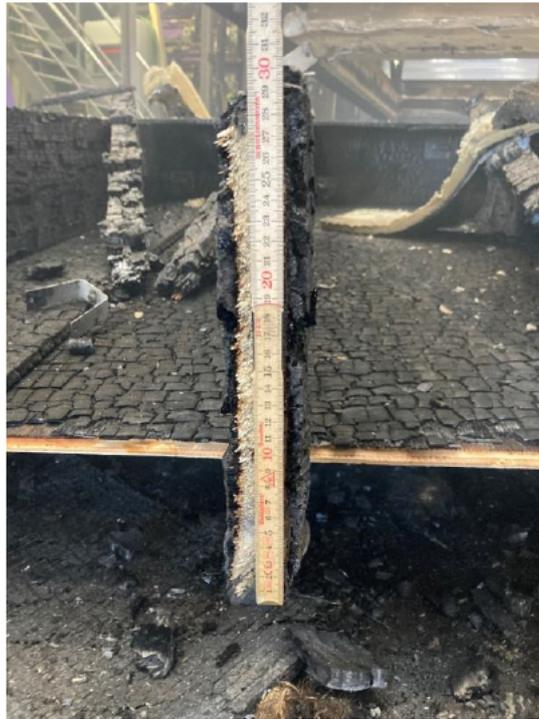
Photo No. 28 The loadbearing beams after the test
