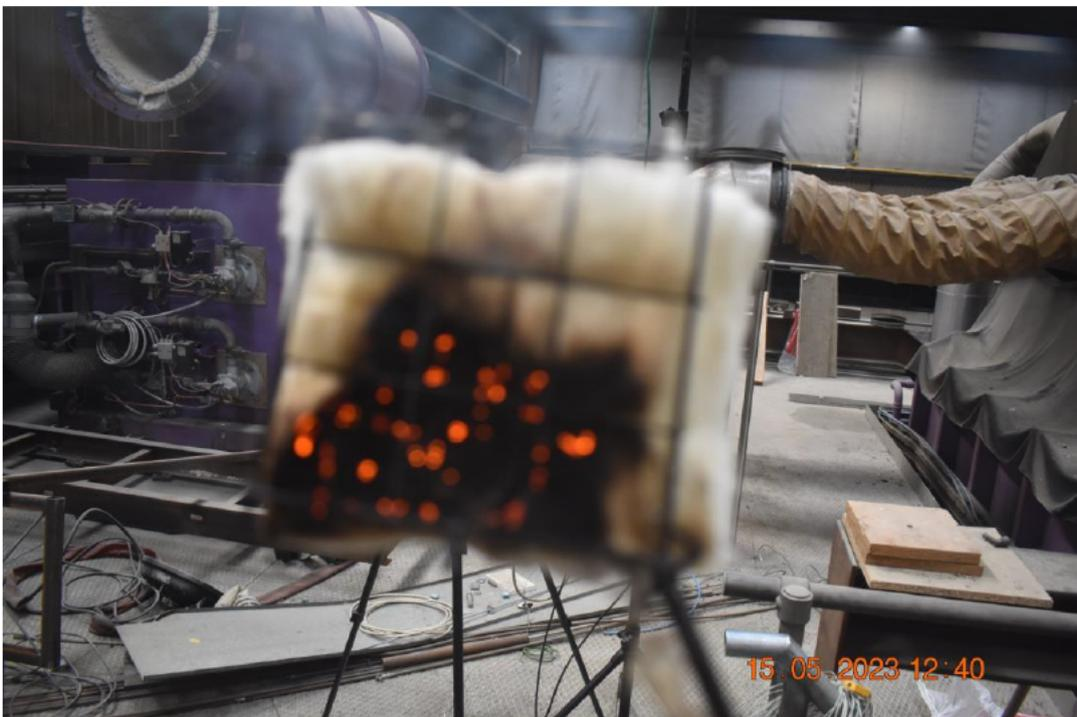
Photo No. 23 Cotton pad test result from unexposed side 60 minutes into testing
