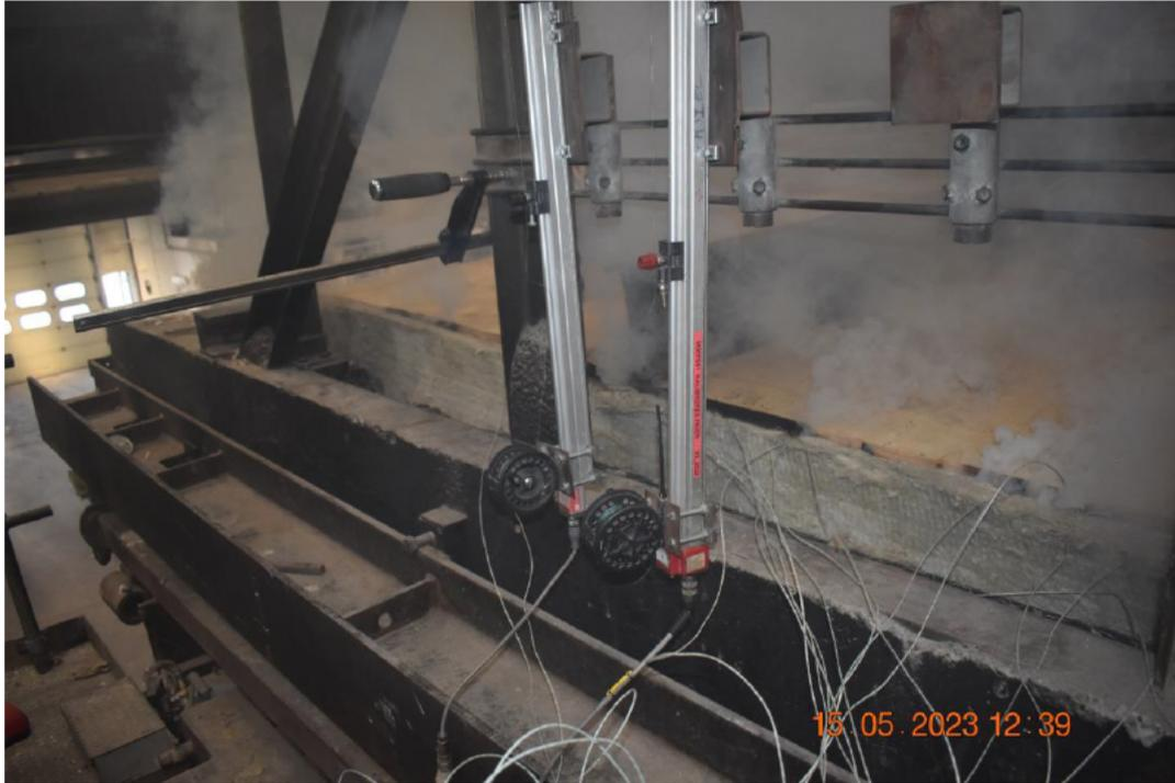
Photo No. 24 Test specimen seen from unexposed side at 60 minutes into testing
