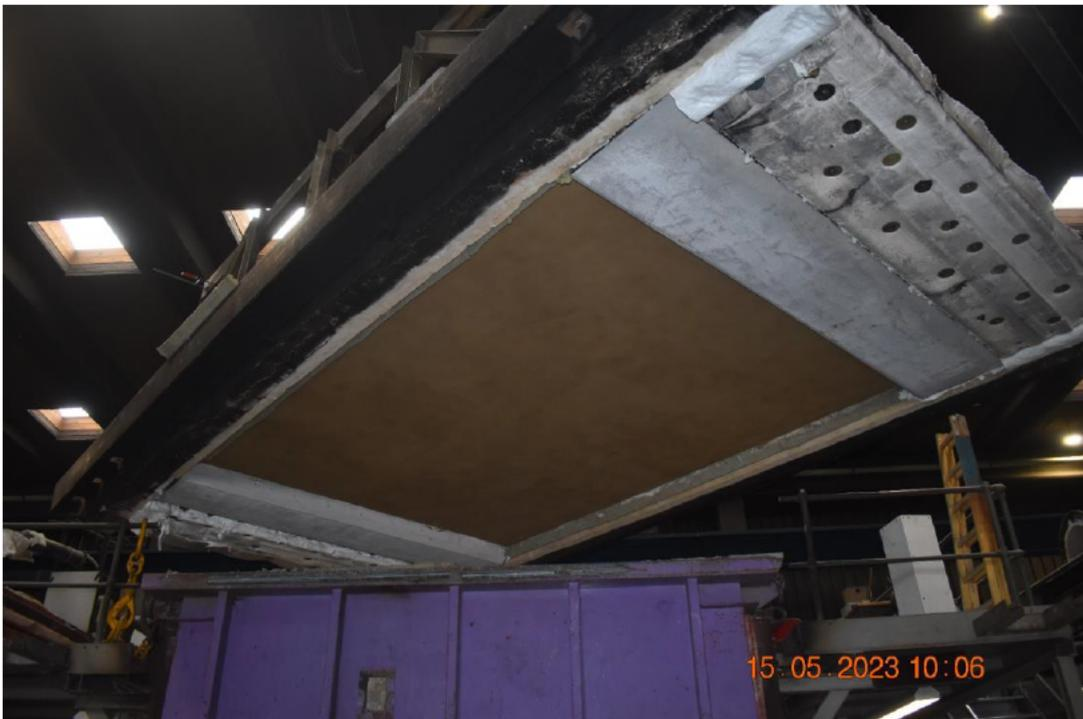
Photo No. 14 Test specimen seen from the exposed side before test
