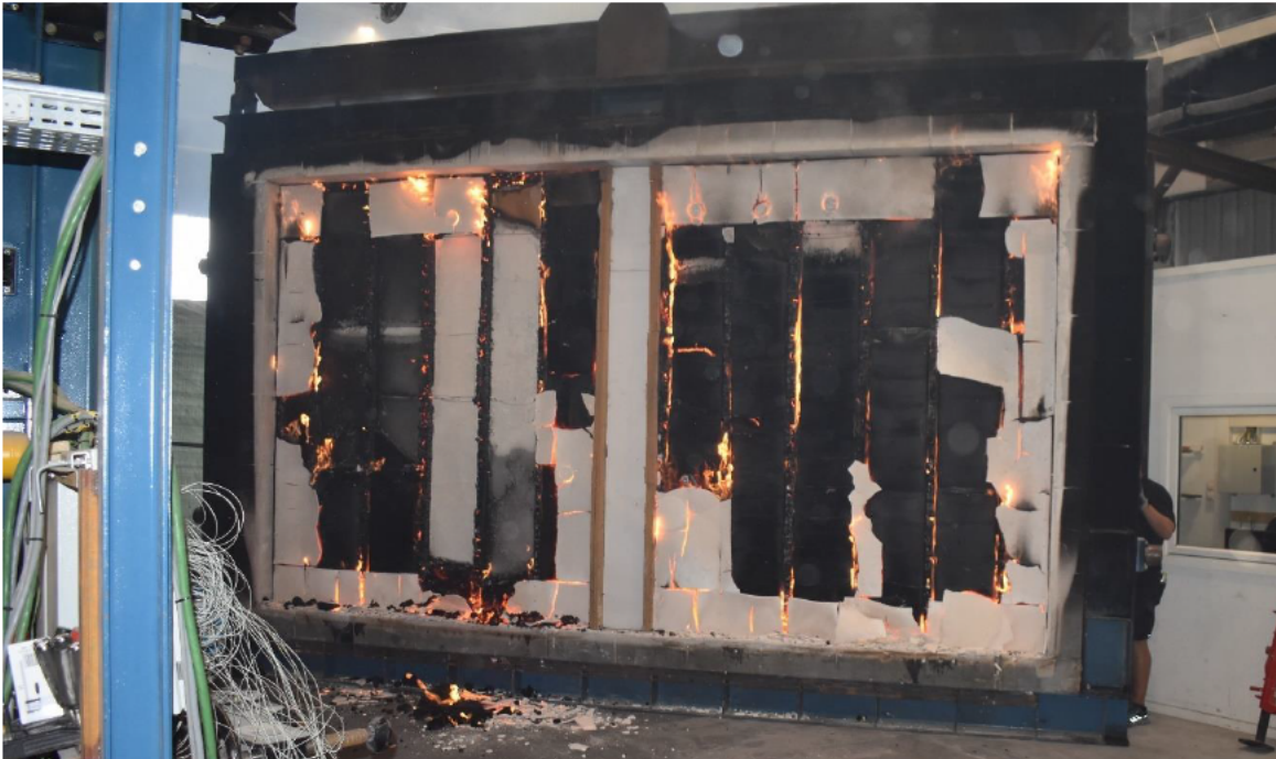
Photo No. 19 Test specimen after test seen from exposed side.
