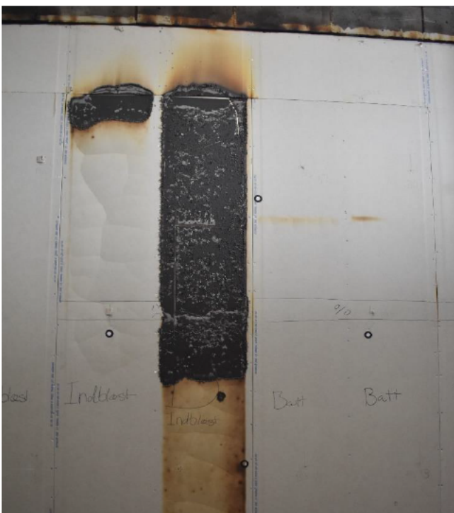
Photo No. 20 Test specimen after test seen from unexposed side.
