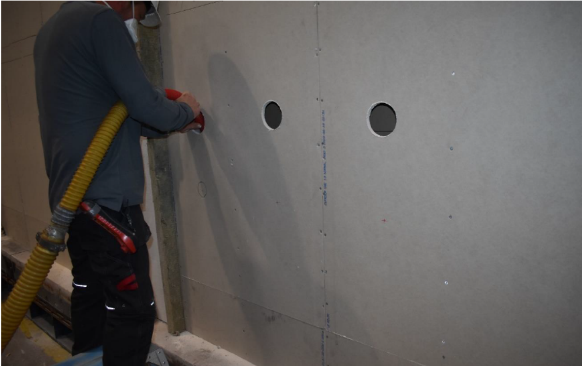
Photo No. 9 Woodfibre insulation being blown in test specimen.
