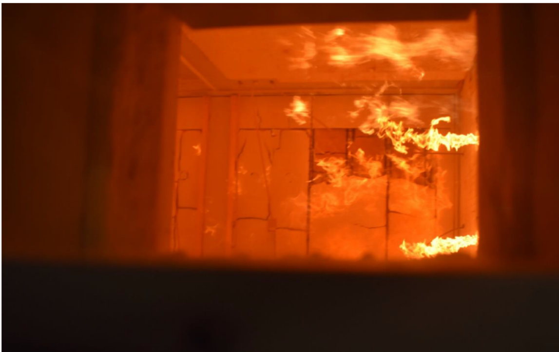
Photo No. 18 Gypsum seen from exposed side.
