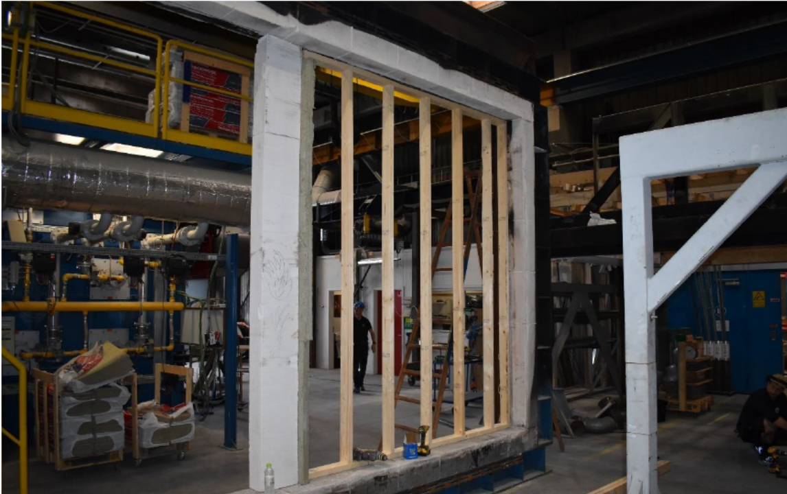
Photo No. 1 Mounting of timber studs in the testing frame.
