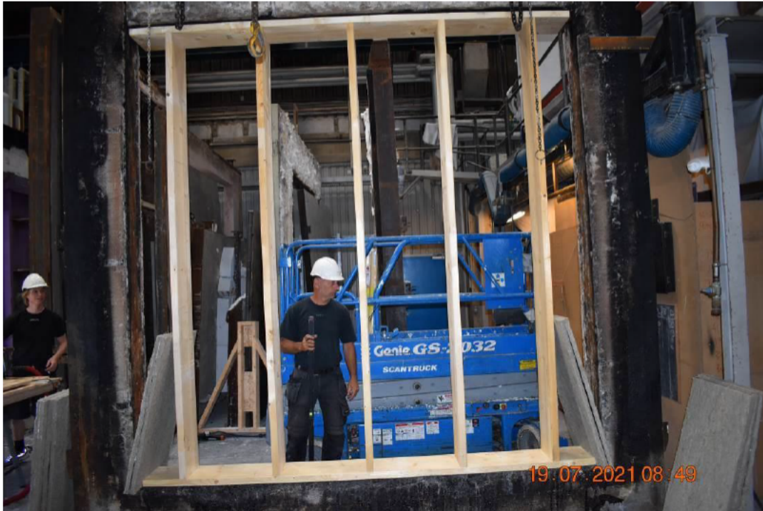
Photo No. 1 Free edge was established along both vertical edges of the test specimen.
