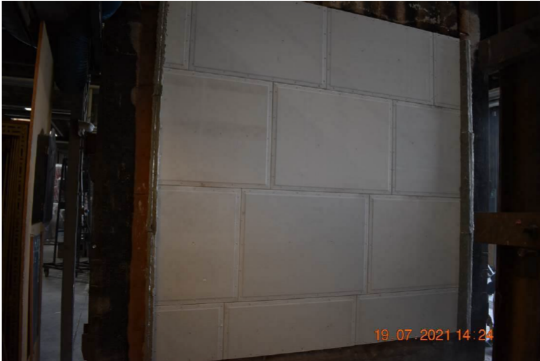
Photo No. 5 Finished layers of the fibre gypsum boards on the unexposed side.
