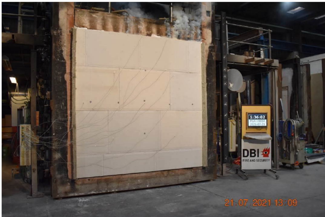
Photo No. 16 Test stopped, 96 minutes into the test
