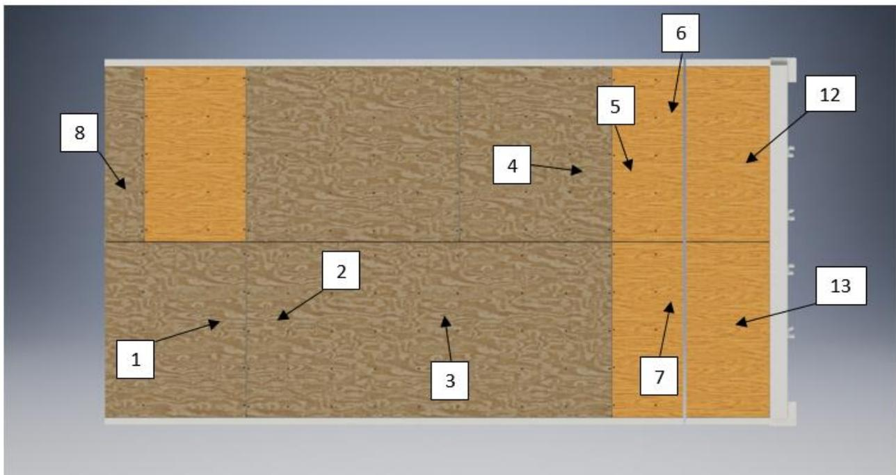
Figure 10 – sampling location on the container floor
