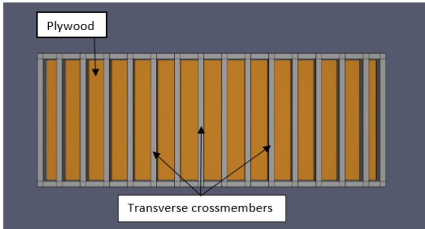
Figure 30: Container understructure
