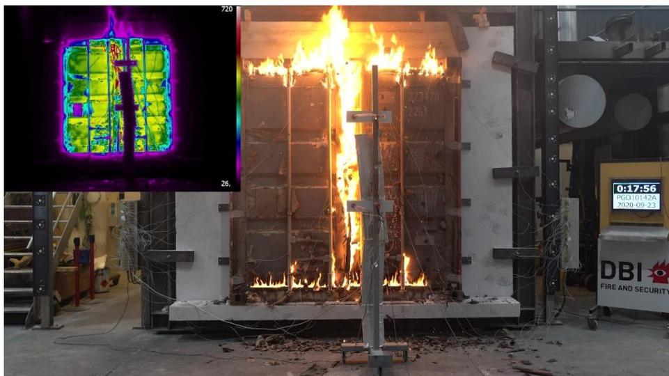
Figure 23 – Ignition of rubbers seal around doors at 17minutes
