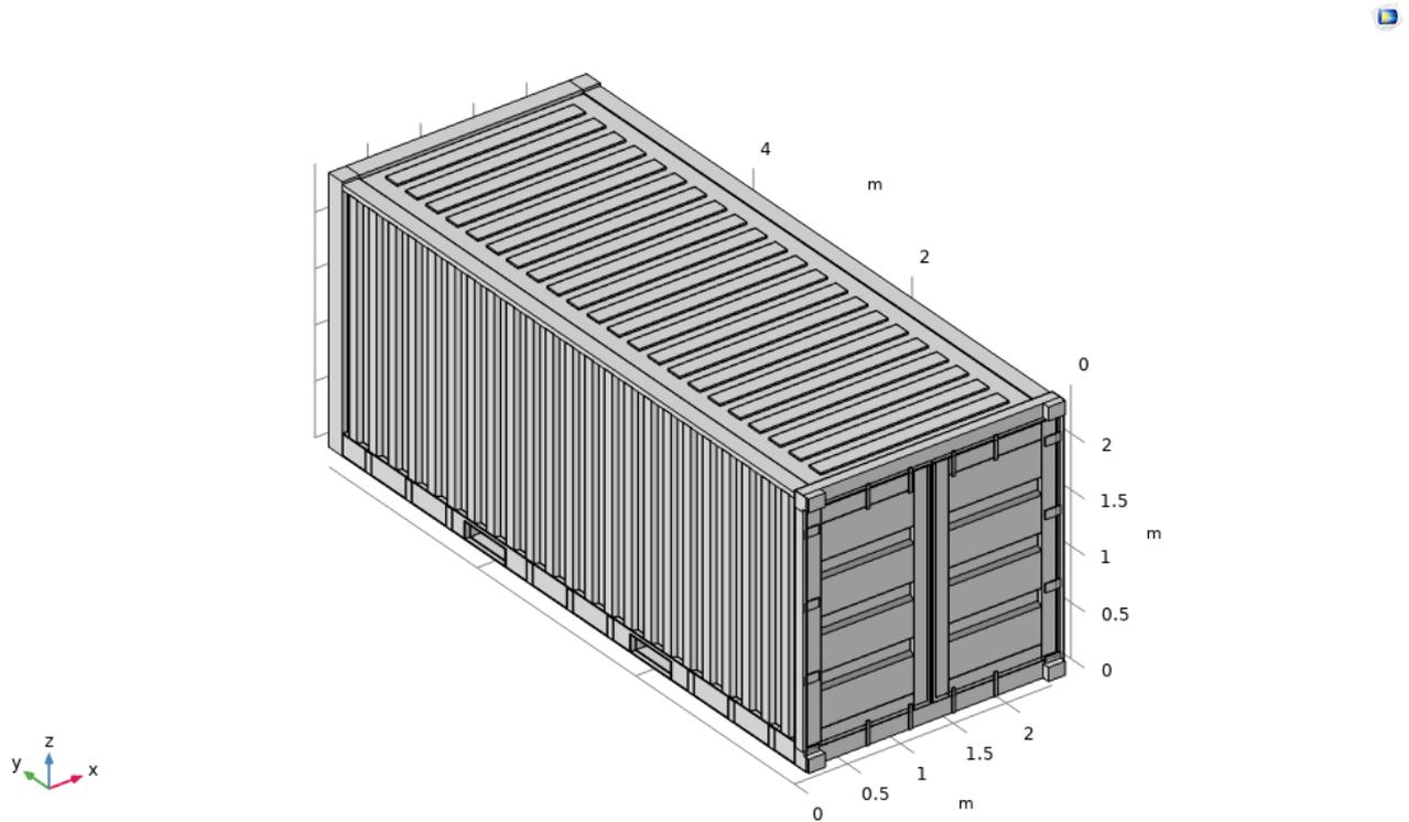
Figure 26 - Geometry of a 20 foot container (snapshot from DBIs model in COMSOL multiphysics)
