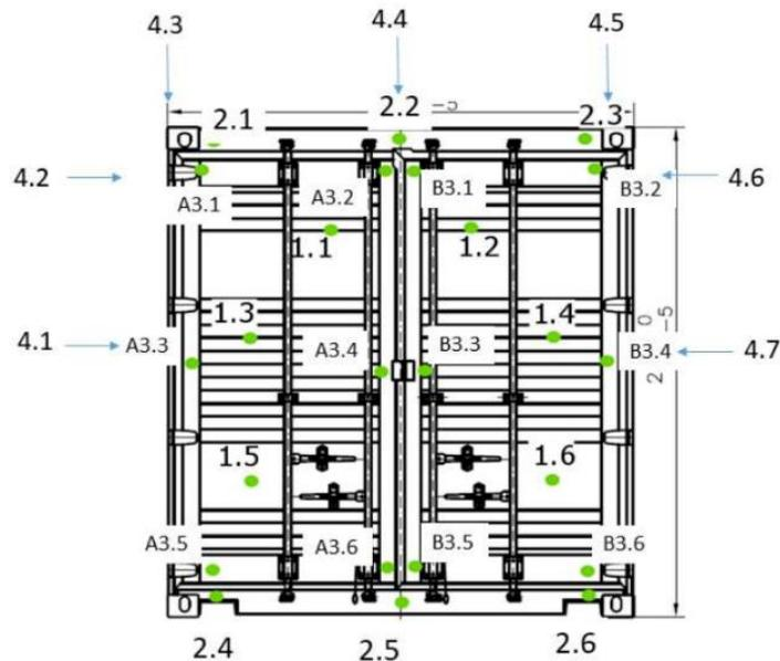
Figure 18 – Thermocouple placement on door
