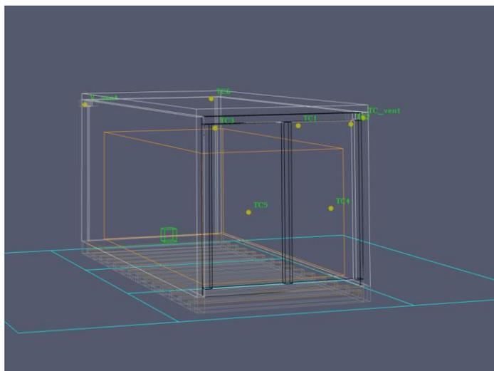
Figure 32: thermocouple locations
