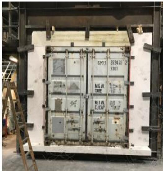
Figure 16 – Door mounted on furnace
