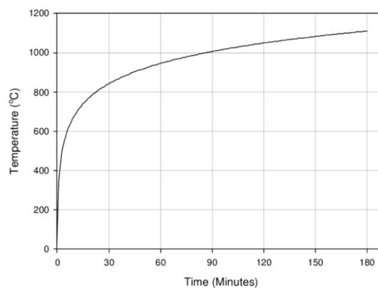
Figure 17 – ISO 834 standard fire curve
